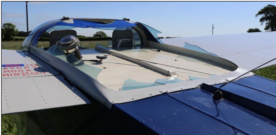
Photo No. 4: Rear Canopy Damage
