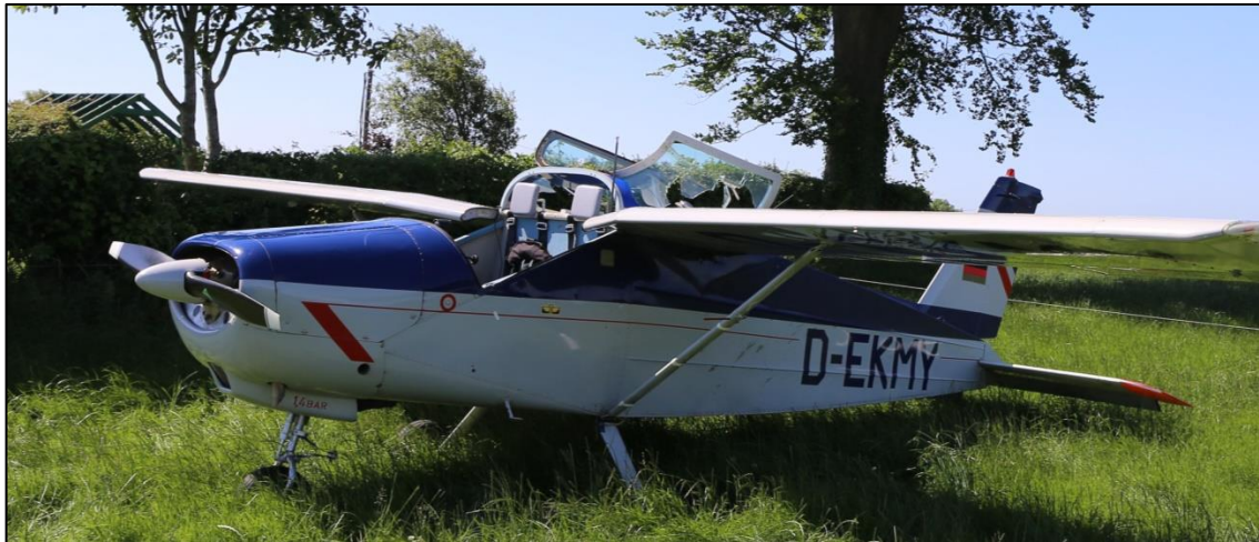
Photo No. 3: Forward Canopy Damage in Open Position
